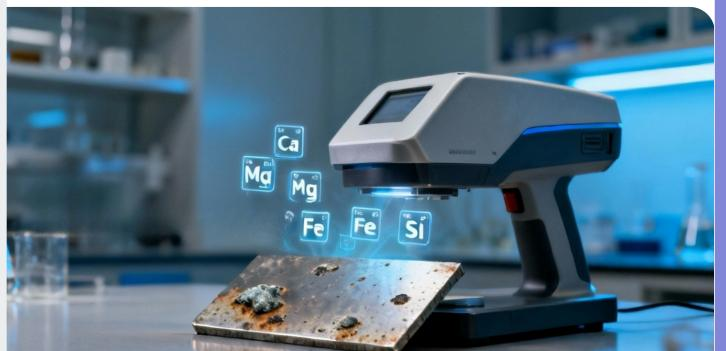
X-Ray Fluorescence (XRF) analysis is a modern method that enables the rapid and reliable detection of elements in solid or liquid samples.
